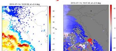
Figure 2. C-band radar De Bilt: left: reflectivity from elevation 0.4 degrees. Right: Rad velocity elevation 2.0 degrees July 14<sup>th</sup> 2010 16.00 UTC
