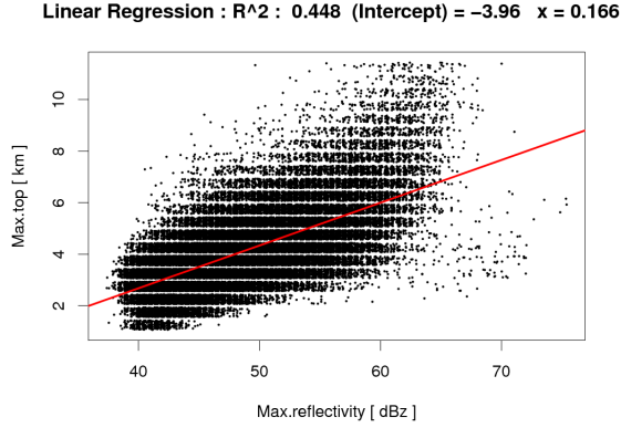
FIG. 7. Scatter plot of maximum echo-top versus maximum reflectivity
